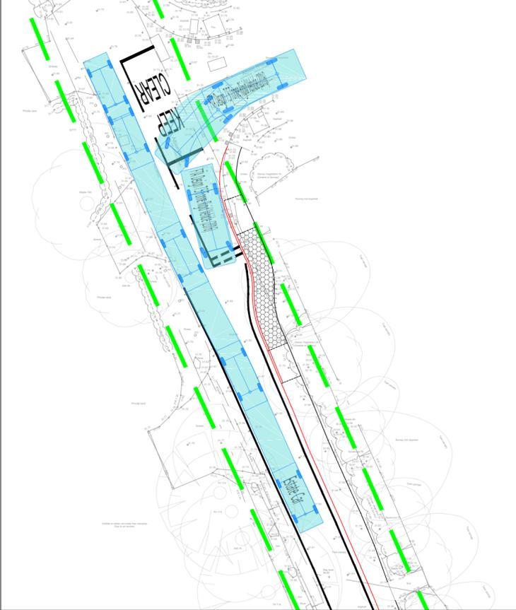
7.5T RIGID VEHICLE TURNING RIGHT OUT OF SITE WITH ESTATE CAR PASSING
