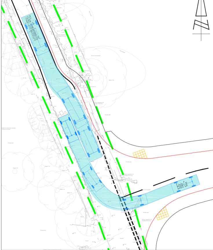
ESTATE CAR TURNING LEFT OUT OF SEYMOUR DRIVE WITH 7.5T RIGID VEHICLE NORTHBOUND
